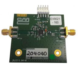
The devices can be used for a wide range of frequencies from 130MHz to 950MHz. The power delivered from the devices depends on the power supply.
